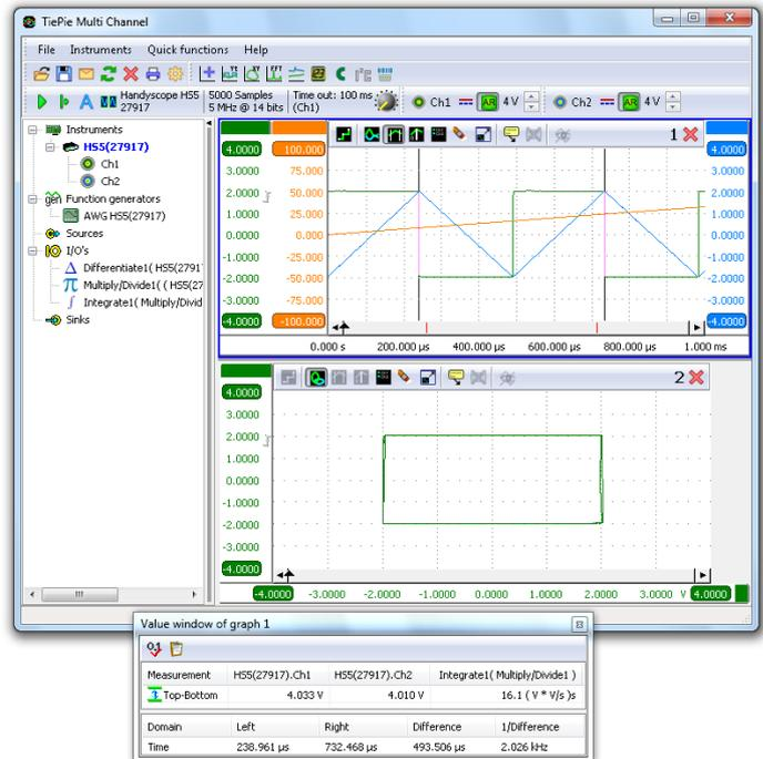
*This measurement determines the area of an XY graph, using multiplying, integrating and differentiating I/O's. The area is indicated in the Value window: 16 V<sup>2</sup>.*
