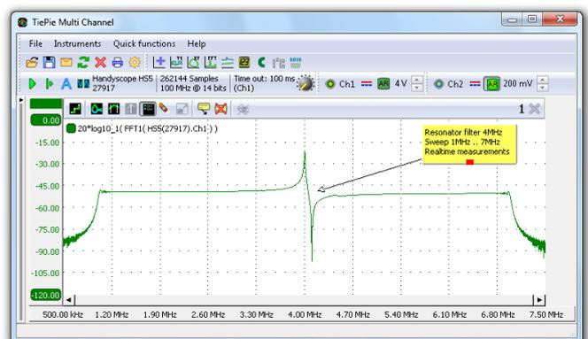
**Very fast 20 MSamples per second streaming Data logger**
