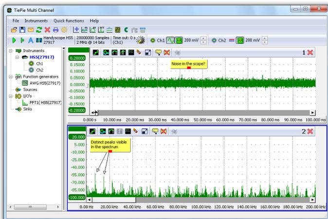
When e.g. measurements are performed on a system that contains switch mode power supplies, the disturbances caused by a power supply are easily detected
