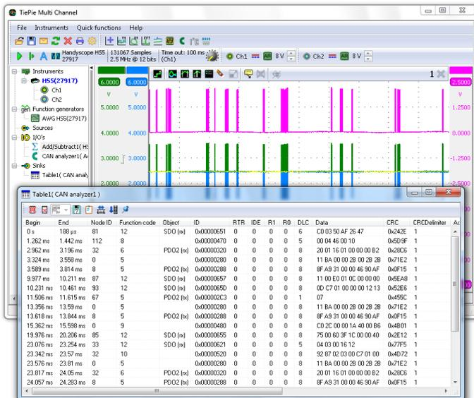
The various serial protocol analyzers of the Handscope HS5 can be used to analyze and debug serial data buses. The data is displayed in an elaborate table with information on the serial data. Locating "wrong" data packets has become very easy. For each developer or service technician this is a welcome option. Protocol analyzers for CAN bus data, I<sup>2</sup>C communication and various other serial data communications are available.
