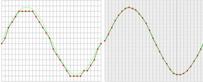
To display a signal measured with the Handyscope HS5 High Resolution oscilloscope at the same level of detail as the standalone oscilloscope, the display can be
