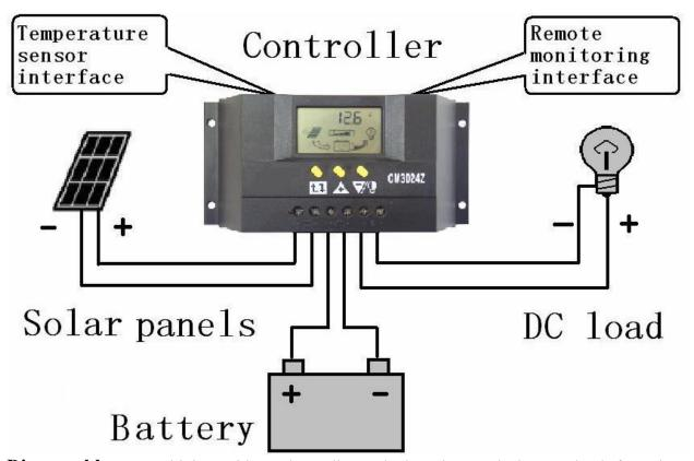
**Disassemble:** To avoid the accident, please dismantle the solar panels, battery, loads from the controller in order.
