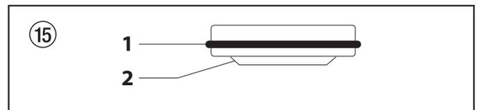
11. Insert lower packing (Fig. 16) with the beveled edge (1) facing upward.
