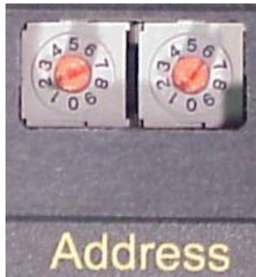
Figure 50: Rotary Switches used to set node address.
