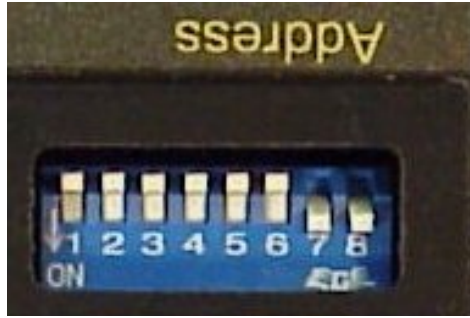
Figure 67: DipSwitch used to set MacID and baud rate
