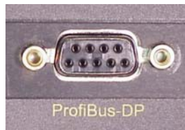
Figure 48: Profibus Connector (from left to right, pin 1 to 5 in bottom row and 6 to 9 in top row)
