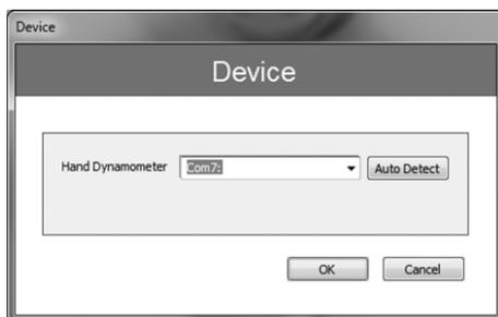
The following message will appear when the DHD-3 Digital Hand Dynamometer is successfully linked with the G-STAR software. Click **OK** to begin using the program.
