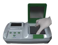
Tear the sealing of a new Graphite Electrode package and take the new Graphite Electrode out of the package. Place the new Graphite Electrode into the anode tank and close the lid of the device.
