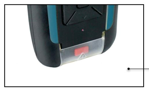
The alert button is under the cover at the bottom of the unit
