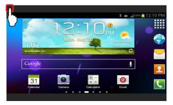
Push in Upper Left corner of the screen to hide/show side bar menu. Use this feature (side bar menu OFF/ side bar menu ON) to reset mouse cursor in the event it's not functioning properly.
