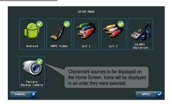
"Factory Backup Camera" source activates factory backup camera. Available only if backup camera was previously activated at least once using "Reverse gear" after vehicle startup. This functionality may not be available for all vehicle models.
