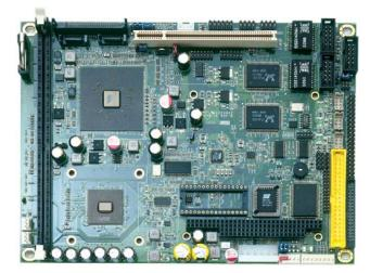
The HS-4610 is a VIA CX700(M) chipset-based board designed. The HS-4610 is an ideal all-in-one embedded engine board. Additional features include an enhanced I/O with CF, CRT/LVDS, TV-Out, dual GB LAN, audio, SATA, 4 COM, USB2.0, and PC/104 interfaces.
