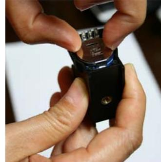
2. Take Battery Holder PCB out of Counter Housing
