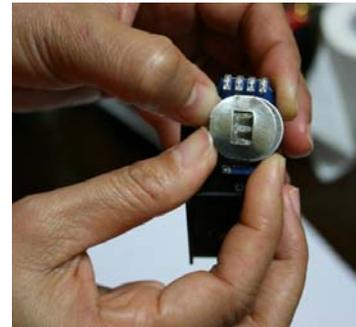
5. Replace with a full battery, insert LEDs to the plastic cover, push back the Battery Holder PCB and screw on Cover of Counter Housing.
