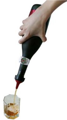
Attached to individual bottles, Skytag wirelessly transmits pour data by the millisecond when the bottle is tilted.
