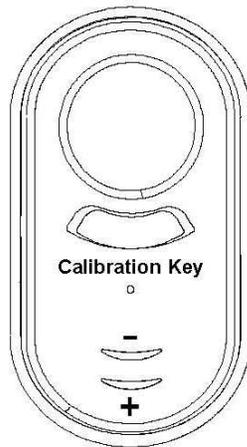
The Calibration Key has the same housing as the Charger and Washing Key. It adjusts the pour rate and refines the pour size. This can also be done through our Skyman software.
