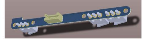
out three MDS6500AL02PS switches to a Hirose DF13-5 connector. A wiring harness splits the connections between the Battery Supervisor PCB (3 wires) and the C&DH board (2 wires).
