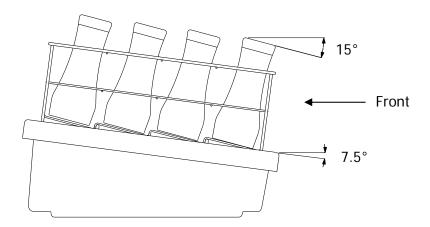
**Important:** Place the compartmented Basket onto the Airack, orientated so that the glasses are tilted towards you, to give the maximum angle.
