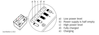
If the battery is turned on and not connected to the scanner:
