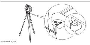
1. Level up the instrument in advance using the re-level functionality in *Cyclone*, assuming that the instrument is correctly adjusted.
