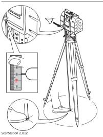
To get an accurate measurement, hold end of measurement tape with your foot on benchmark. Now expand the measurement tape and read height using etched horizontal reference line on unit
