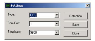
The standard type of connection used is UDS protocol. COM Port 1, and the standard Baud rate is 9600.
