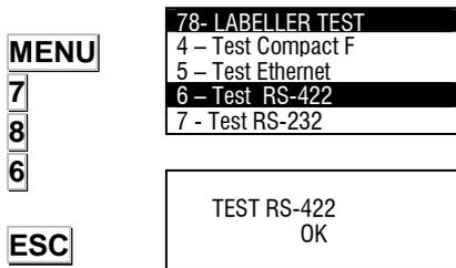
It is possible to make a test of the RS-422 Communications Channel.
