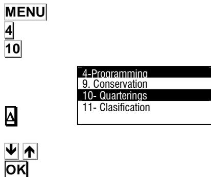
This is designed to automate the labelling of the parts of an animal. Up to 100 cuts with up to 100 lines (parts) each can be programmed.
