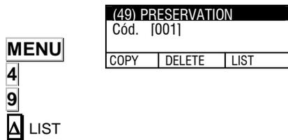
It is possible to view on-screen the list of conservation texts programmed on the labelling machine. To do this, proceed as follows:
