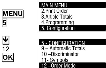
From the initial screen, Press **MENU** to enter in the main menu, press the key **5** to enter in the Configuration programming and the key **↓** until reach Configuration 12, (it is also possible by pressing the key **→** to pass to the second screen of the menu and pressing **↓** until reach Configuration 12) Orders mode and pressing the key **OK**.
