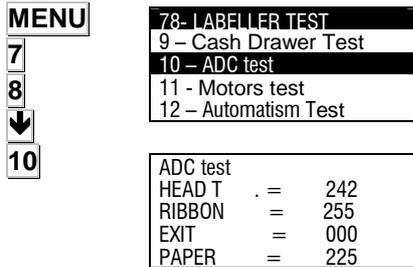
From the main screen press **MENU** to enter in programming mode, select **7** Test and press **8** to select Labeller Test.
