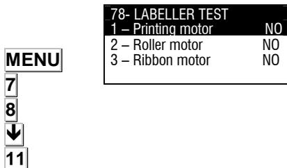
From the main screen- press **MENU** to enter in programming mode, select **7** Test and press **8** to select Labeller Test.
