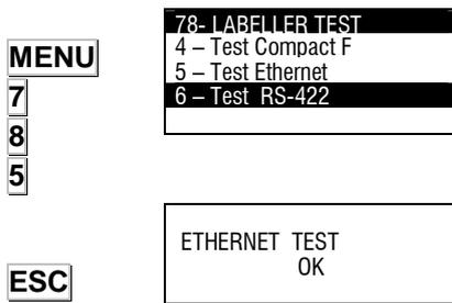
It is possible to make a test of the Ethernet Communications Channel.
