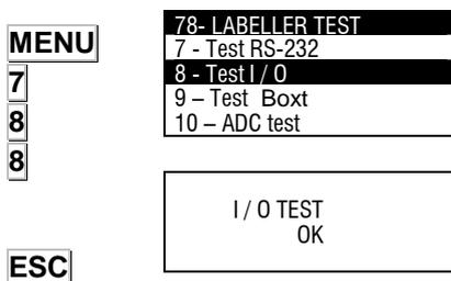
From the main screen press **MENU** to enter in programming mode, select **7** RS-232 Test and press **8** to select Labeller Test.
