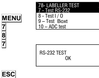
It is possible to make a test of the RS-232 Communications Channel.
