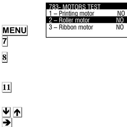
From the main screen press **MENU** to enter in programming mode, select **7** Test and press **8** to select Labeller Test.
