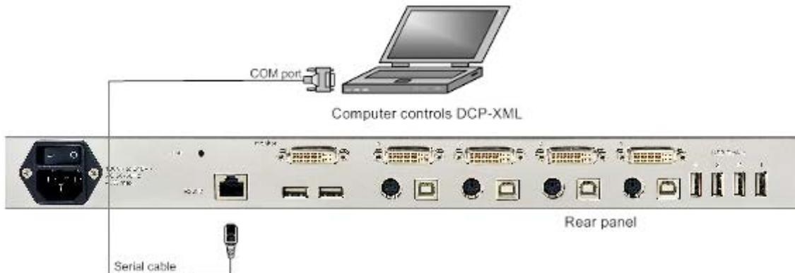
Use the serial cable to connect the COM port of the Windows computer with the serial port of your QuadraVista 2.
