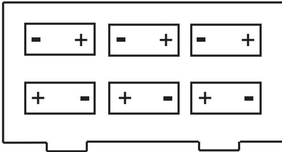
Figure 2-2. Battery Installation
