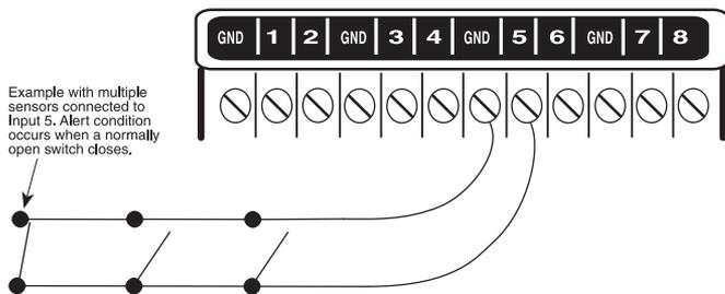
**Figure 2-9. Multiple Normally Open Sensors**
