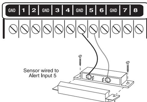
**Figure 2-6. Sensor Connected to an Alert Input**
