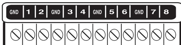
Figure 2-5. Alert Inputs
