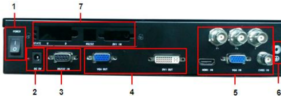
Figure 3.2 CK4L-1000 Mini Full Color LED video processor Rear panel diagram
