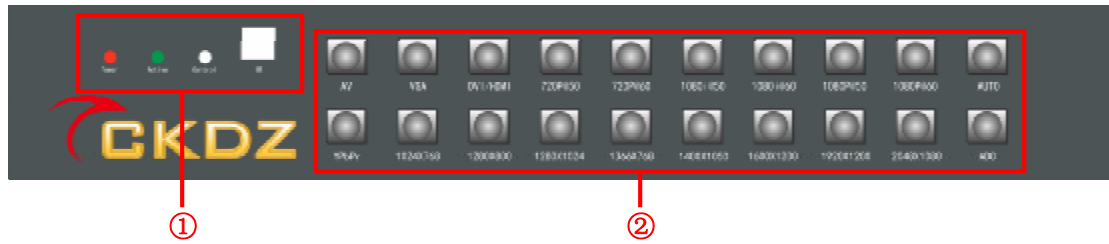
Figure 3.2 CK4L-1000 Mini Full Color LED video processor Front panel diagram
