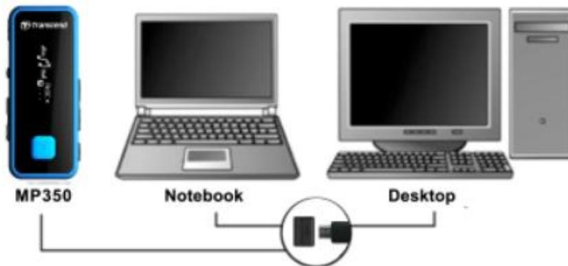
2. When connected to a computer the MP350's screen will display a "CONNECTED" message, indicating that files can be loaded onto the player.
