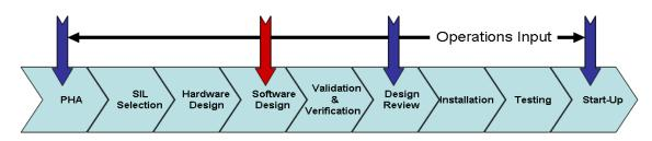
Figure 1: Operations Input into SIS Design
