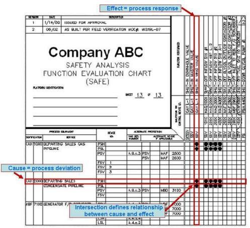
Figure 2: Cause and Effect Diagram
