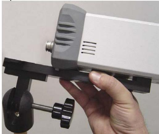
Attaching PMM DR-01 Double ridged Antenna.
