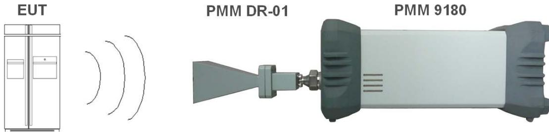
**Fig. 3-1** Radiated emission test setup – PMM DR-01 Vertically polarized with PMM 9180
