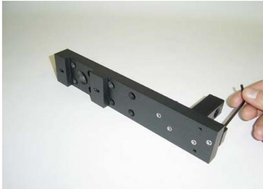
Mounting the Antenna Holder on PMM 9180
