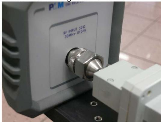
Change the PMM 9180 polarization from horizontal to vertical or vice versa and tighten the knob completely.
