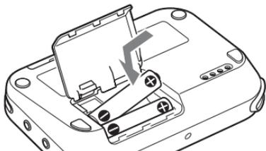
Be sure to insert the batteries with the **+** and **-** ends in the right position.
