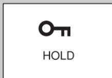
“HOLD. Slide HOLD Switch to Activate.” appears if you press any button when the HOLD function is activated.
