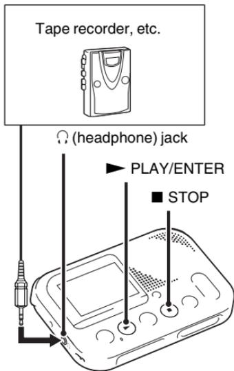
You can record the sound of the memory card recorder with other equipment. Before you start recording, we recommend you make a trial recording first.
