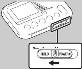
Slide the HOLD•POWER switch in the direction of “HOLD.” “HOLD” will appear for approximately 3 seconds, indicating that all the button operations are disabled.
