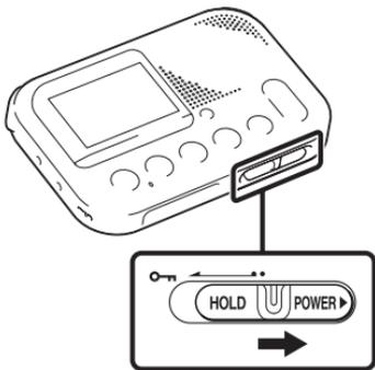
Slide the HOLD•POWER switch in the direction of “POWER” and keep it there until the opening animation appears.
