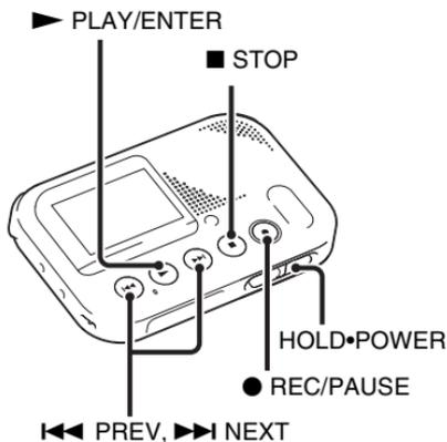
You can record a new file by pressing the ● REC/PAUSE button. Recorded files are not erased. The recording level is set automatically. You can also review the latest recording file by just pressing the ► PLAY/ENTER button without the rewind operation.
