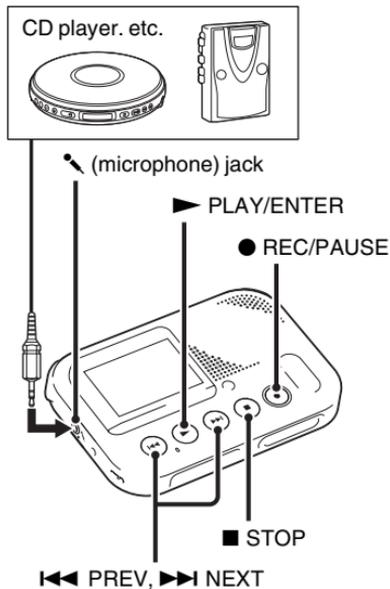
You can make MP3 files without using the computer by recording sound from other equipment connected to the memory card recorder.
