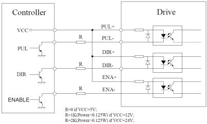
R must be connected to control signal terminal.
