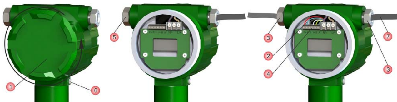
Figure 2.11 - Electrical connection of the flowmeter
