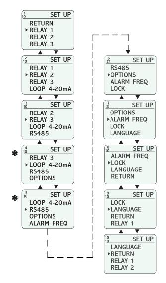
Is the main menu from which is possible to set up all the parameters involved in the equipment. It is accessed from the status screens when pressing the button "Enter". It is also possible to arrive by chosing the succesives options RETURN included in whichever of the rest of menus or screens.
