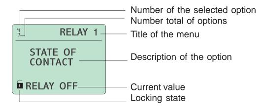
Once placed on the screen that shows the parameter we want to modify its value, press ● in order to access to the screen for changing the value.
