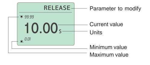
Once placed on the screen that shows the parameter we want to modify its value, press • in order to access to the screen for changing the value. Since the modification is done digit by digit and not like a complete value, the first digit at left remains blinking. Press  $\blacktriangle$  to modify the value and • to validate it and to advance to the following digit. When the last digit becomes validated the preceding screen is visualizated again.
