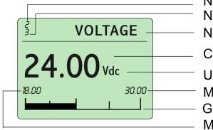
Number to current screen Number to total screens Name of the magnitude Current value Units Maximum limit Graphical bar Minimum limit
