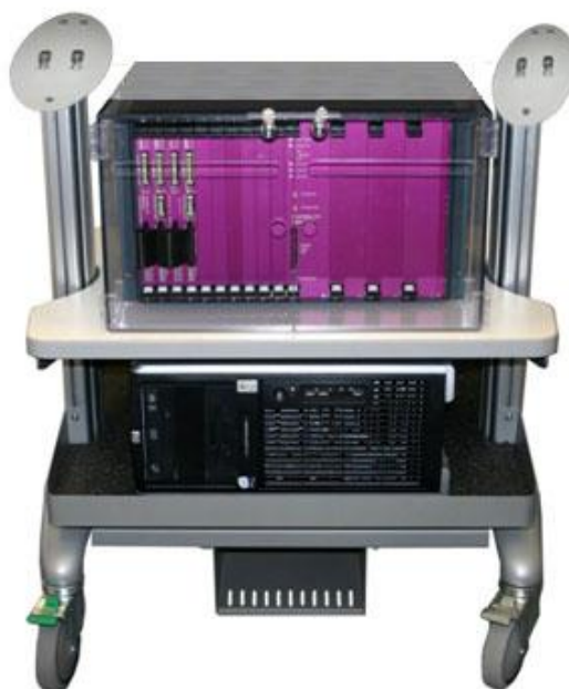
Figure 6-7 Isolation Cart with Digital Lynx and Computer
