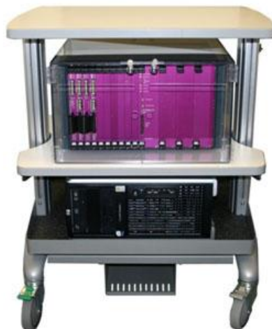
Figure 8-2 Isolation Cart with Digital Lynx and Computer (monitor stand not shown)
