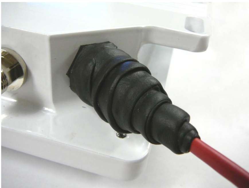
Figure 7.6.1: Properly taped Ethernet adapter
