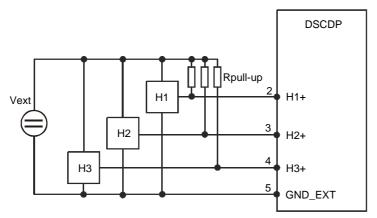
An external pull-up (resistor) must be added per sensor. A resistor of 1.5 k $\Omega$  (1/4 W) must be used if Vext is equal to +15VDC. If the user needs to supply the Hall effect sensor with another voltage, please contact ETEL to define the value of the resistor.
