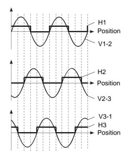
The digital Hall effect sensors (H1, H2 and H3) must be connected as shown below:
