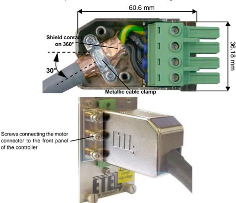
**Remark:** The cable's radius of curvature must be taken into account to adjust the distance between the front plate of the controller and the cabinet.
