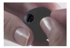
Use the battery tool to push the cap down and turn it clockwise until the dot on the cap aligns with the top dot on the tracker. You'll feel a little click when the door is closed correctly.
