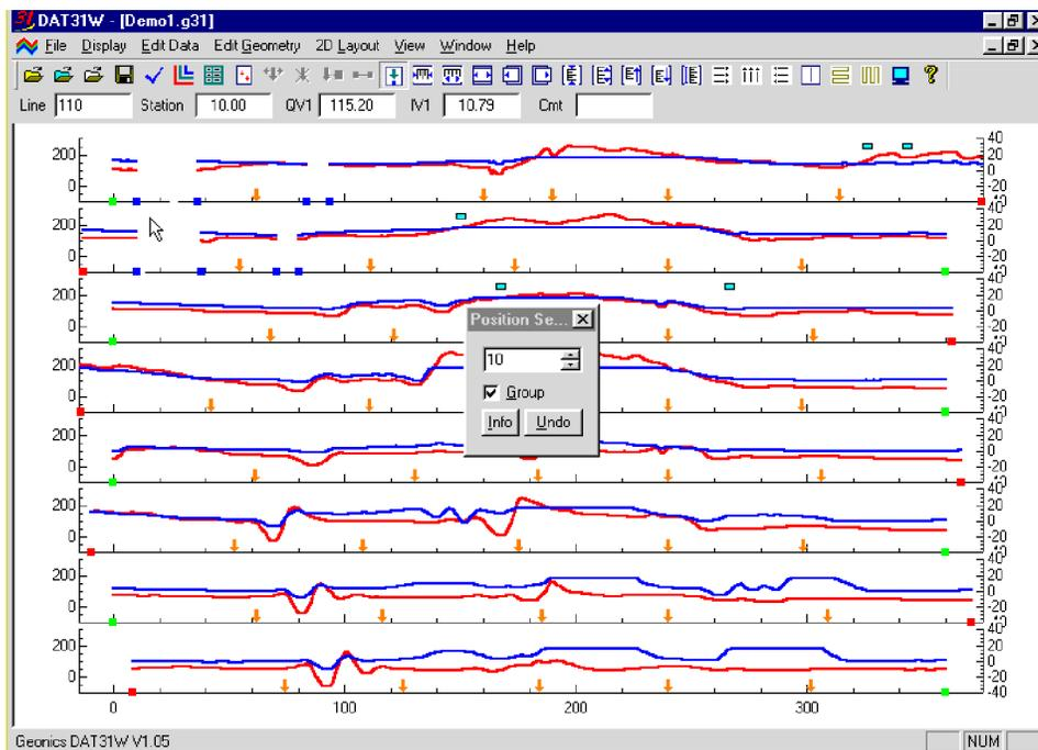
Figure 6.18: DAT31W screen after positioning group of selected end stations (compare Figure 6.17)
