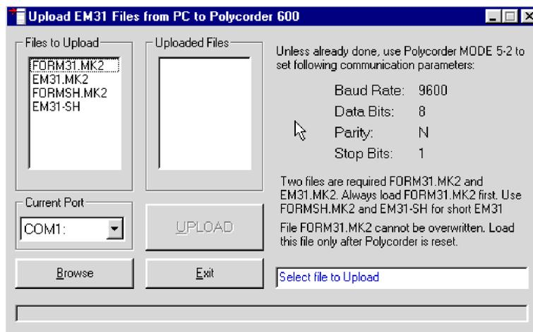
Figure 3.2: Upload EM31 Files from PC to Polycorder 600 window
