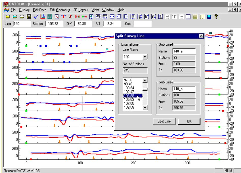
Figure 6.8: Profile View display before survey line split
