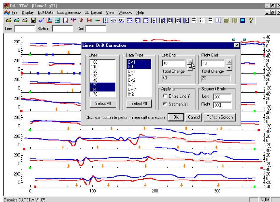
Figure 5.11: The DAT31W screen during Linear Drift Correction of Line Segments
