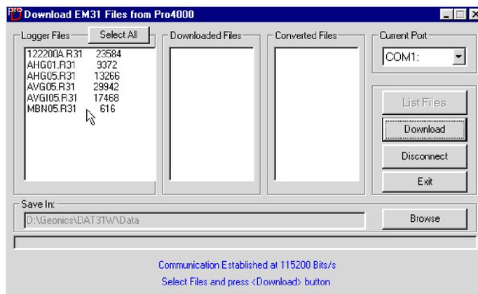
Figure 3.17: List of files available in Pro4000 for Download in Download EM31 Files from Pro4000 window
