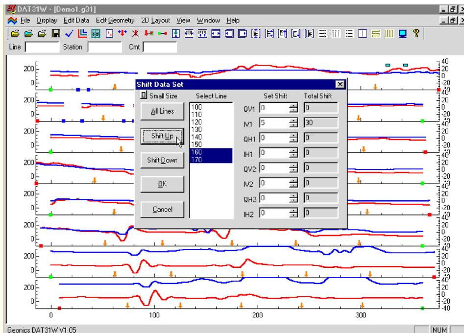
Figure 5.8: DAT31W screen during Shift Data procedure
