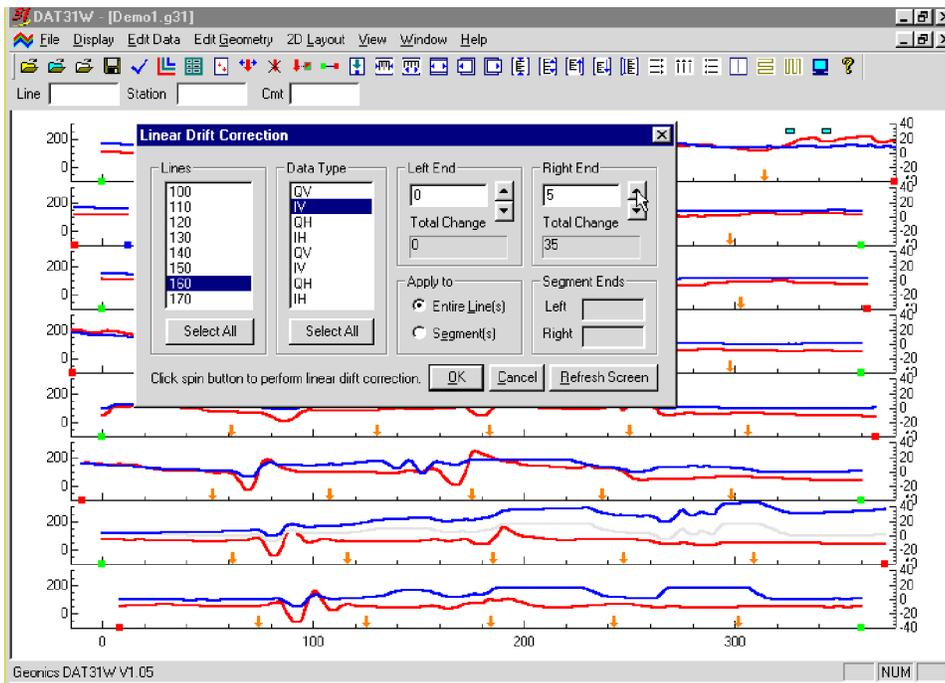
Figure 5.10: The DAT31W screen during Linear Drift Correction for the Entire Line
