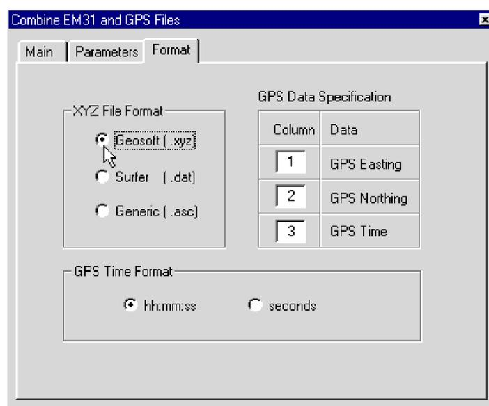
*Figure 8.7: Format page in the Combine EM31 and GPS Files window*
