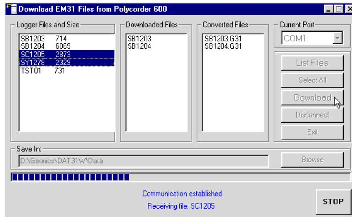
**Figure 3.11: Download EM31 Files... window during data transfer**
