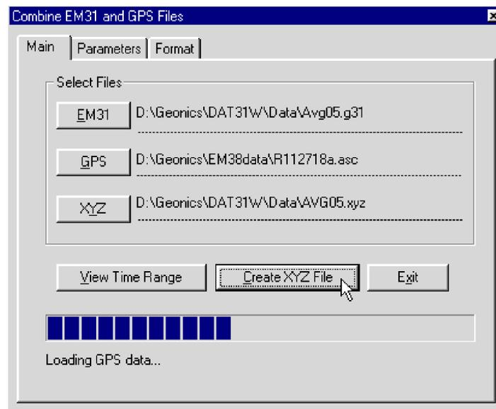
Figure 8.10: Combine EM31 and GPS Files window during reading data files and creating output XYZ file
