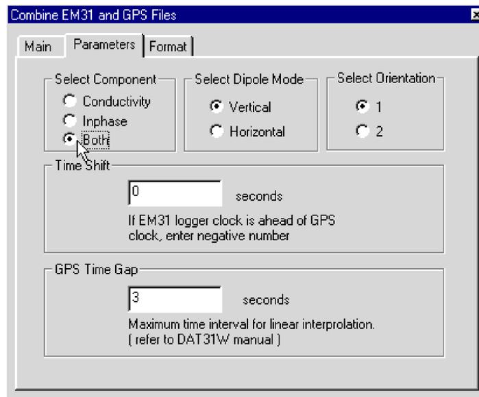
**Figure 8.6: Parameters page in the Combine EM31 and GPS Files window**
