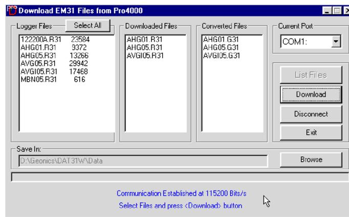
*Figure 3.21: Download EM31 Files from Pro4000 after downloading selected files is completed*
