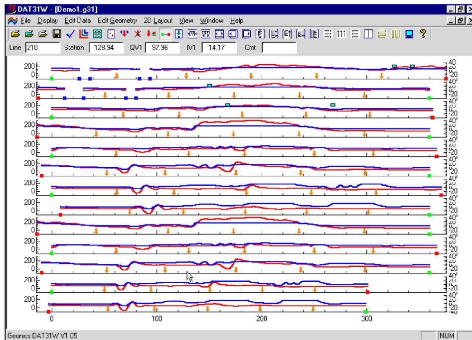
Figure 4.7: DAT31W screen with content of three files in one window
