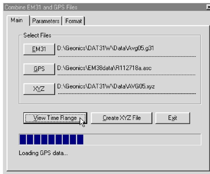
**Figure 8.8:** *Combine EM31 and GPS Files window during reading of EM31 and GPS files*
