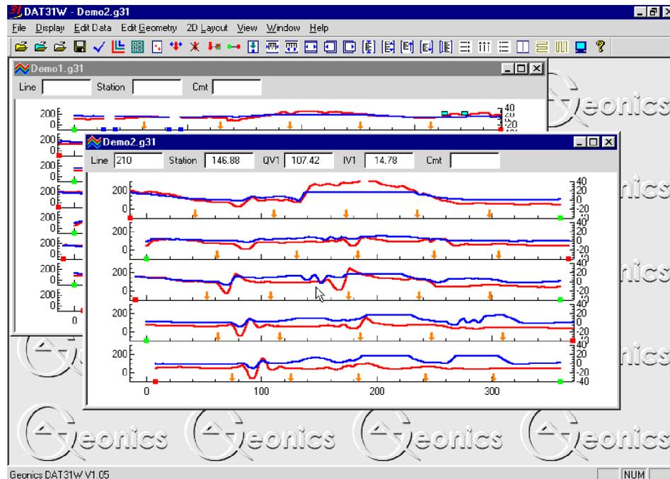
Figure 4.6: DAT31W screen with stacked profiles in two windows
