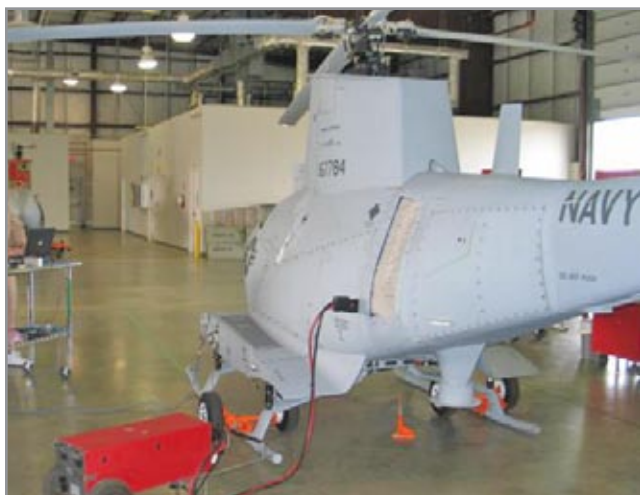
Figure 3.10.5 Starting Fire Scout with TI3500 GPU-24
