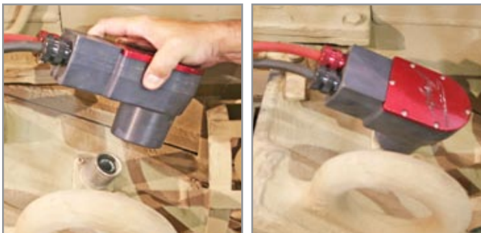
Figure 3.10.3 Attaching NATO DC Power Cable to vehicle
