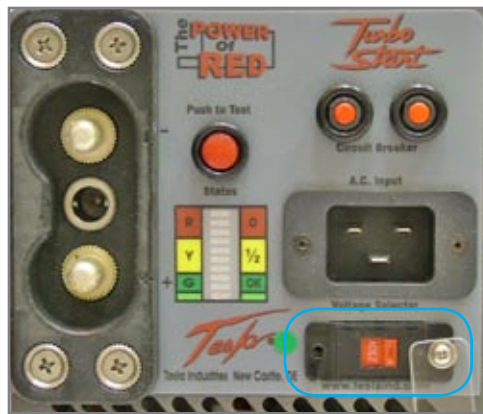
Figure 2.9.1 Input Voltage Selector Switch (outlined in blue)
