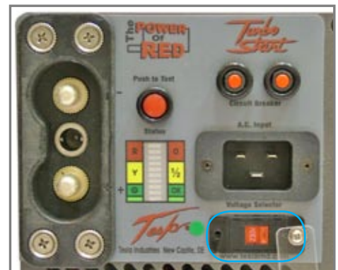
Figure 1.3.4 – T13500 GPU-24 Input Voltage Selector Switch
