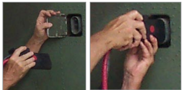
Figure 3.10.4 Attaching an Aviation DC Power Cable to aircraft
