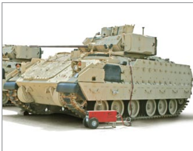
Figure 3.10.6 Starting Vehicle with TI3500 GPU-24
