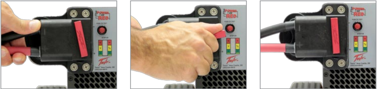
Figure 3.10.1 Attaching DC Power Cable to TI3500 GPU-24
