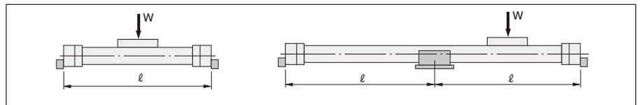
**Caution:** If the support span exceeds 4000mm [157.48in.] with  $\phi 63$  [2.480in.], or 5000mm [196.85in.] with  $\phi 80$  [3.150in.], adapters must be installed in the middle regardless of the load.
