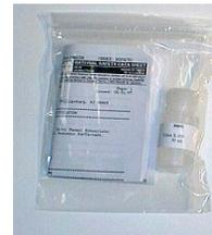
Conductivity cell cleaning solution (Triton-X)
