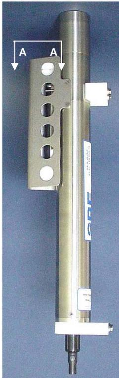
Before each deployment, clean the bleed hole with 0.4 mm diameter wire, 13 mm long (0.016 inch diameter wire, 0.5 inches long) (you can use #26 AWG wire), and blow through it to ensure it is open. A clogged bleed hole can trap air, preventing the pump from functioning properly; this will affect the data quality.
