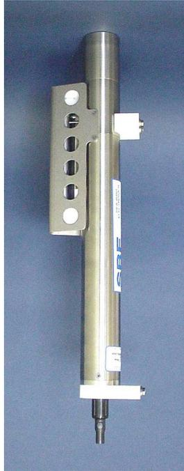
For most applications, deploy in orientation shown (connector end down) for proper operation
