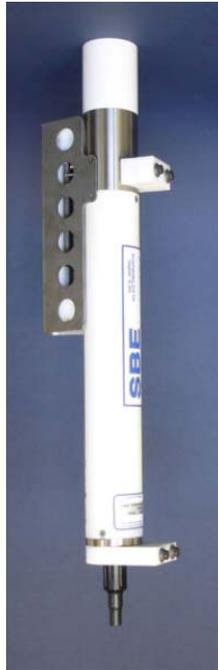
For most applications, deploy in orientation shown (connector end down) for proper operation – see *Optimizing Data Quality / Deployment Orientation in Section 4: Deploying and Operating MicroCAT*
