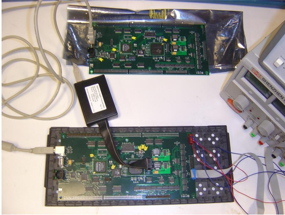
Figure 5.1: Real-Time Controller Board Prototype
