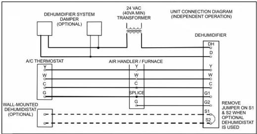
**Damper Connection.** If an optional damper(s) is used in the discharge/return duct, this may be controlled by the dehumidifier. See "Unit Connection Diagram - Independent Operation", above for connection details. When connected as shown in the above diagram, the dehumidifier provides only the switching interface for the damper(s). Power for these devices must be provided with a separate transformer (not provided), not from the transformer located in the dehumidifier.
