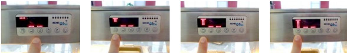
The **primary heating** (heat from below) can be set in three power levels by pressing the
