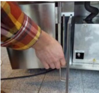
For some units with a substructure, there are two slide-ins for the removed hinged doors. The doors can be stored there when operating the unit with the operating side open.
