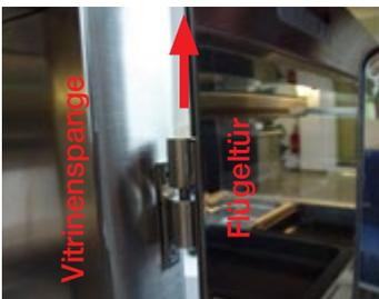
The hinged doors have a mirror coating on the inside. They can be removed in order to provide more space in peak times and for removing the items. We recommend their removal only when the glass pane on the customer side is closed; otherwise the temperature and humidity on the inside of the heated display case cannot be maintained.
