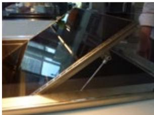
When closing the primary hotplate, make sure that it is controlled with the centrally placed grip and guided down until it reaches the home position.
