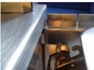
As soon as the bracket has been removed, the mirror can be unhooked from the right side.
