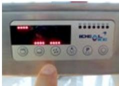
After being switched on, the controller always shows power level NEUTRAL for all heat sources. The unit will not heat up. The light can be switched ON and OFF.
