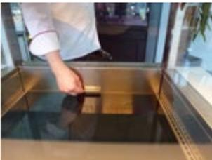
Lift up the primary hotplate from the operating side using the centrally position grip. The panel remains open due to the gas damper.
