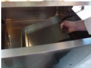
The water tray for generating the humidity is found on the inside of the well. Remove the tray.
