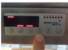
By pressing push button
