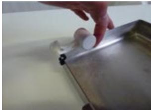
After removing the water tray, carefully remove the float. Now you can conveniently clean the inside of the well in addition to all the parts removed from the heated display case.
