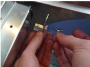
Unscrew the wing screw and remove the bracket that becomes free.
