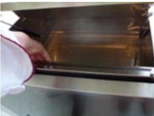
Take out the steam deflector plate with the slide controls.
