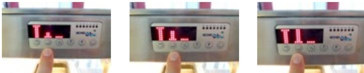
The **supporting heat** (from above) can be set in three power levels by pressing the
