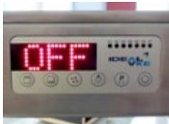
When a heated display case of the BASIC Line is connected to the power mains, „OFF“ must always appear in the display. That way you can also be sure that the unit is connected to the power supply.
