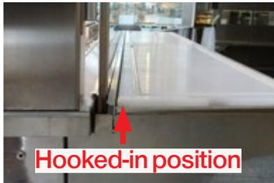
The mirror is folded up. The cutting board support can now be pushed in until it snaps into place. Afterwards, reinsert the cutting board. Make sure that the bracket points towards the front of the unit.
