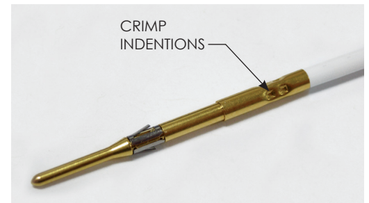
Figure D. Correct location of the crimp divots.
