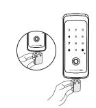
While brining a 9V battery into contact at the external power contact section on the front ass'y, bring the card key or the key tag into contact at the door lock or enter the secret code.
