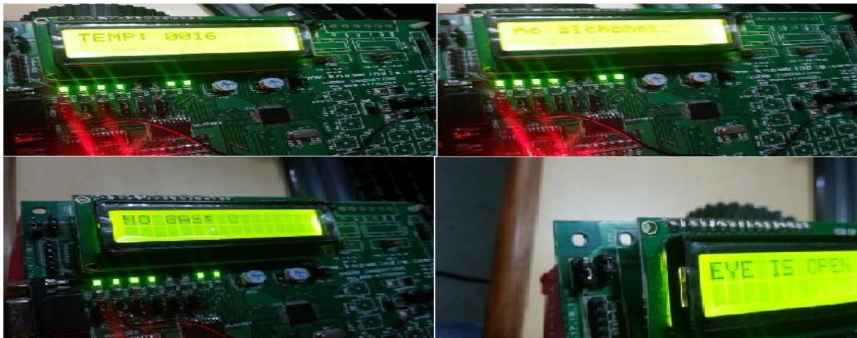
Fig 8: Vehicle monitoring system with Temperature, Gas, Alcohol, PIR, and Eye blink Sensors
