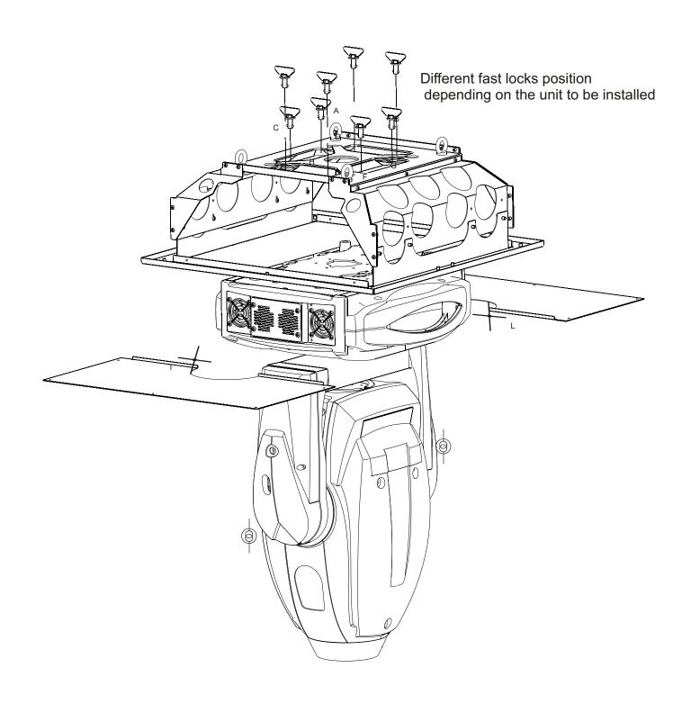
Place in position the 2 metal covers by using the 5 fixing screws each.
