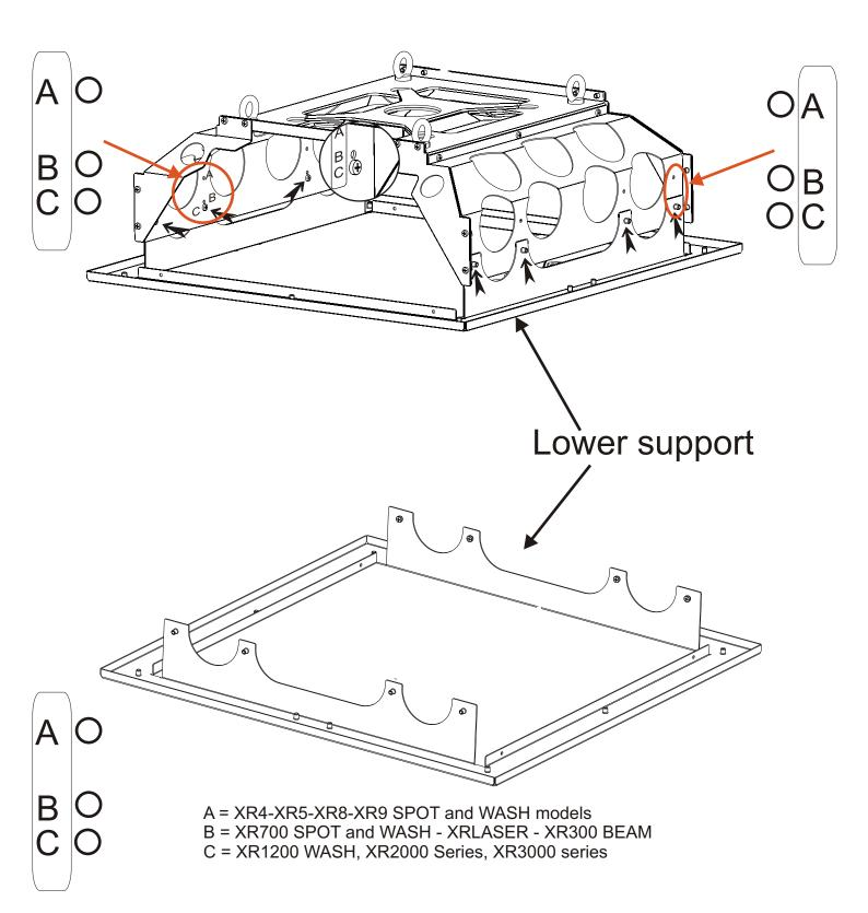
Complete assembly to be fixed on the ceiling
