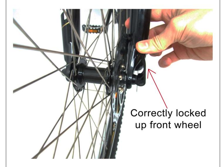
Please note what the correct and incorrect set up of the front axle
