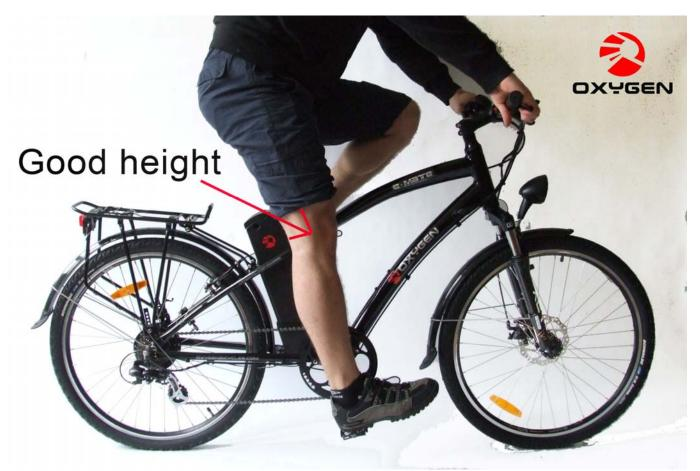
While adjusting the seat height please note that each seat post has the safety marking on the seat pillar. Please do not exceed the border of safety in any circumstances. The markings on the seat pillar always need to be hidden in the seat tube and never exposed above it. Seat post adjusted above its acceptable limits may cause the personal injury as well as the damage to the frame.
