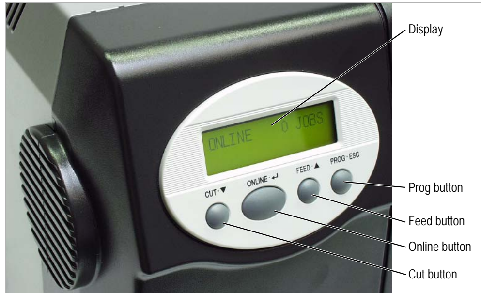
[8] Control panel of the AP 7.t
