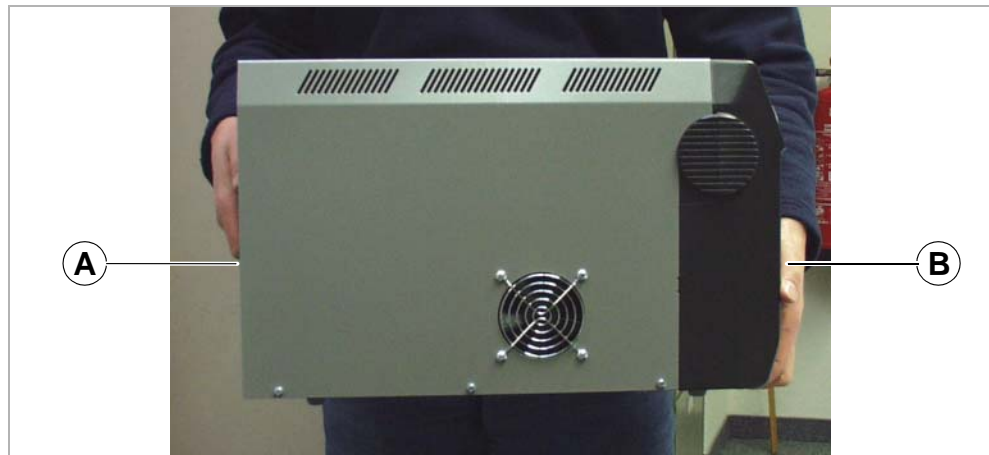
[1] Carrying the AP 7.t safely (A: back – grab by the feed slot, B: front – grab by the base plate).
