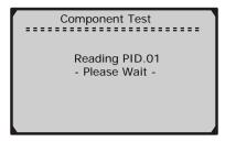
3) From the **Component Test** Menu, use the **UP/DOWN** scroll buttons to select the test to be initiated.
