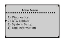
2) From the **DTC Lookup** menu, use the **N** button to move to the desired character, use ≈ or ≈ arrow buttons to change selected digit/character and press **Y** button to confirm.
