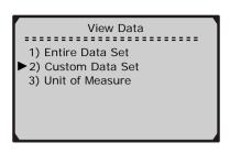
7) Use the **UP/DOWN** scroll buttons to move up and down list, and press the **Y** button to select or deselect data parameters to view. Selected parameters are marked with solid squares.
