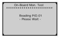
3) From the **On-Board Mon.Test** menu, use the **UP/DOWN** scroll buttons to select the test to view and press the **Y** button.
