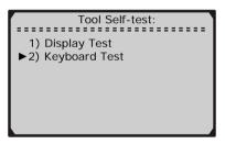
2) Press any key to start test. When you press a key, the key name should be observed on the display. If the name does not show up, then the key is not functioning properly.
