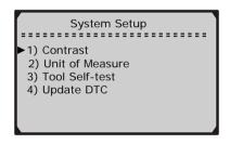
**From the Main Menu:** Use the **UP/DOWN** scroll buttons to select **System Setup**, and press the **Y** button. Follow the instructions to make adjustments and settings as described in the following setup options.
