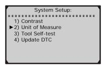
2) From the **Unit of Measure** menu, use the **UP/DOWN** scroll buttons to select the desired unit of measurement.
