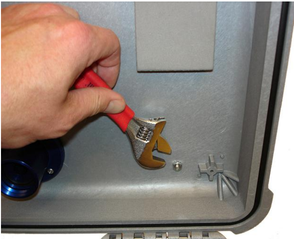
Figure 4: Remove Waterproof Bolt Assemblies from Heat Shield Mount Locations
