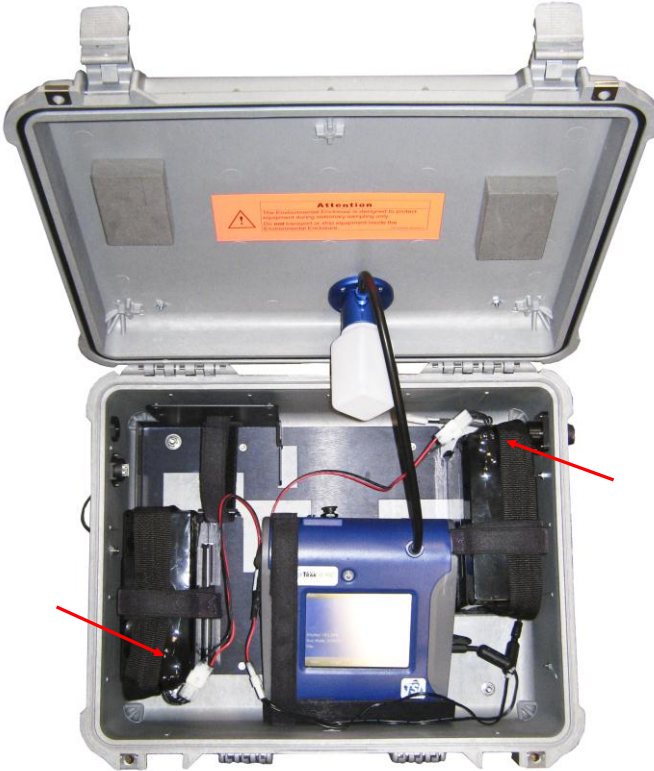
Figure 22: Install the Dual Battery Pack System
