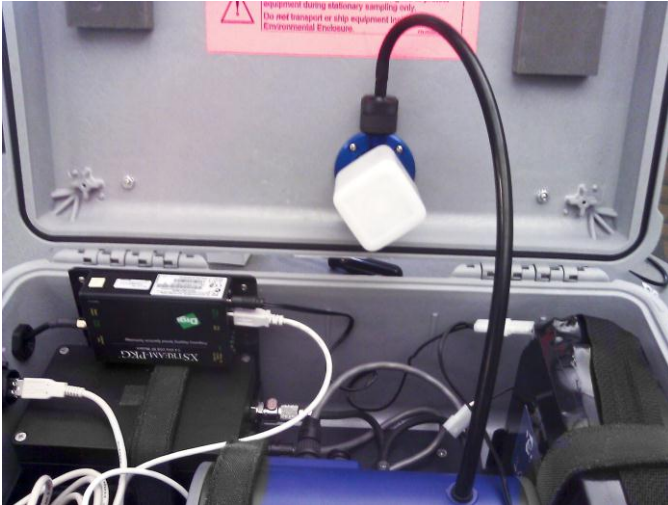
Figure 35: Connect Sample Tubing
