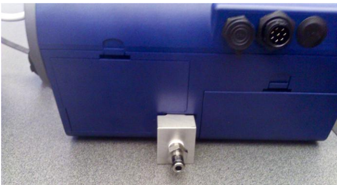
Figure 28: Install Exhaust Adapter
