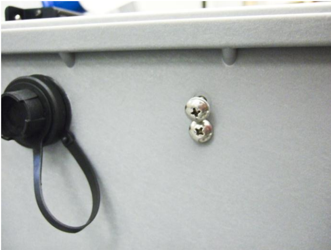
Figure 15: Remove Two Screws to Secure Antenna
