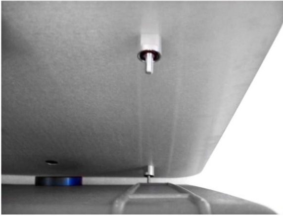
Figure 5: Attach Heat Shield to the top of the Enclosure
