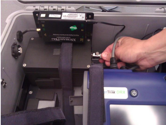
Figure 31: Connect External Pump Flow Tube
