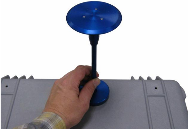
Figure 3: Thread the Inlet into the Inlet Ring
