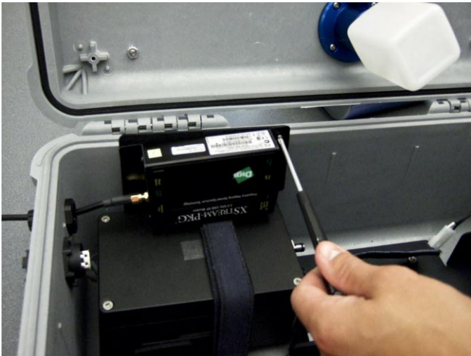
Figure 13: Attach Radio Modem to Bracket
