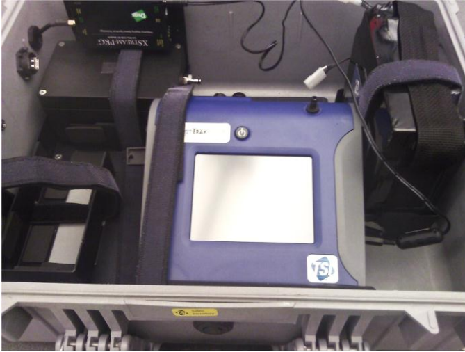
Figure 27: Install DustTrak Monitor in the Bracket
