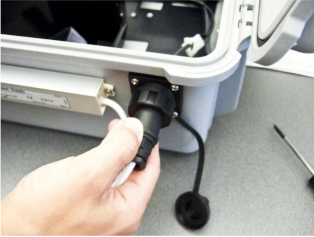
Figure 25: Connect Adapter DC Cable to Enclosure
