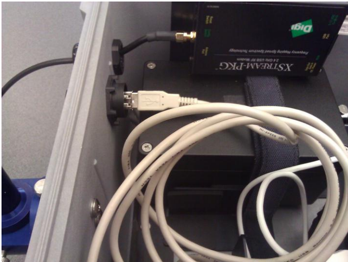
Figure 34: Connect USB Cable for Pass-through
