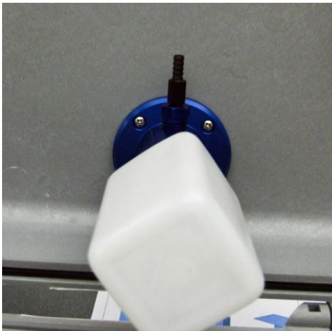
Figure 7: Install the Water Trap Bottle
