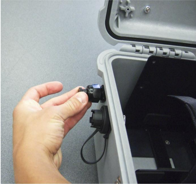
Figure 10: Remove the Antenna Cable Fitting Plug
