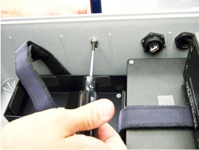
Figure 16: Attach Antenna Mounting Bracket to Enclosure
