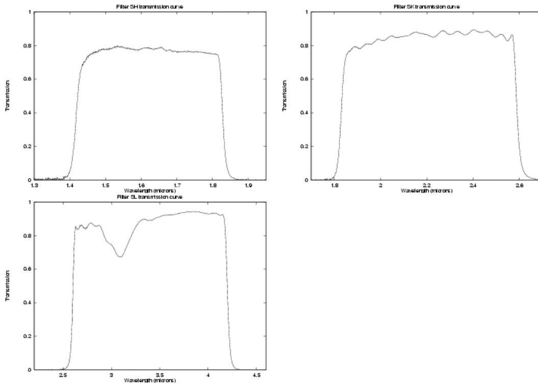
Figure 19: Filter curves for order sorting filters
