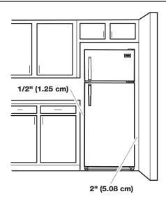
To ensure proper ventilation for your refrigerator, allow for a 1/2" (1.25 cm) space on each side and at the top. When installing your refrigerator next to a fixed wall, leave 2" (5.08 cm) minimum on the hinge side (some models require more) to allow for the door to swing open. If your refrigerator has an ice maker, allow extra space at the back for the water line connections.
