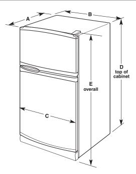
Dimensions "D" and "E" include rollers extended 3/4" (1.9 cm)
