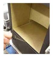
2. The bottom plate is gently lifted out of its position with a wide slotted screwdriver
