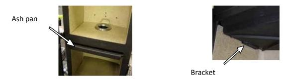
The ashes are swept on to the ash pan and disposed of. Replace the ash pan in its position in the lower combustion chamber again.
