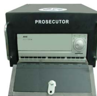
Figure 6 : DVR in Vault
