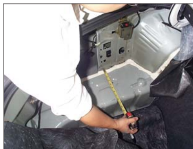
Measure 3-7/8" out from the edge, use 17/64 metal drill bit to drill a hole.
