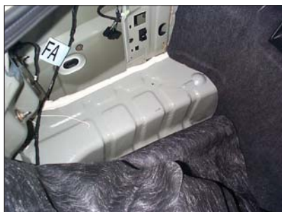
Partially remove carpet from work area.
