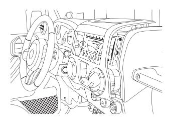
2 Remove the knee cover panel and extract 2 x 7mm screws located to the right and left sides of the steering wheel column.
