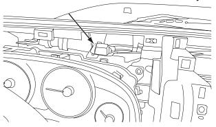
5 Plug the OBDII connector on to the OBDII port below the driver side dash and run the extension to the radio cavity.
