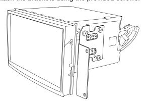
5 Run the key harness through the top-left side of X009 headunit. Mount the X009 headunit using 4 x 7mm factory screws.
