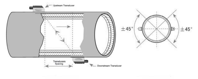
Z-method is commonly used when the pipe diameter is above 200mm.
