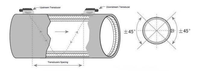
V-method installation is the most widely mode for daily measurement with pipe inner diameters ranging from 15 mm to 200 mm. It is also called reflective mode.
